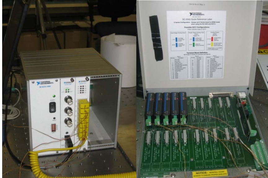
Figure 27: National Instruments (17) Multi-input Type-K Thermocouple Interfaces
