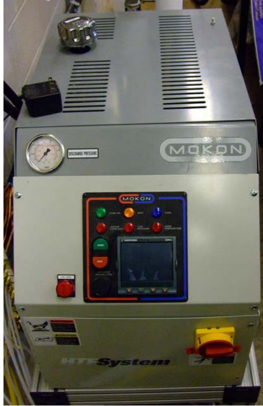
Fig. 13. Mokon heat transfer fluid pump and heater
