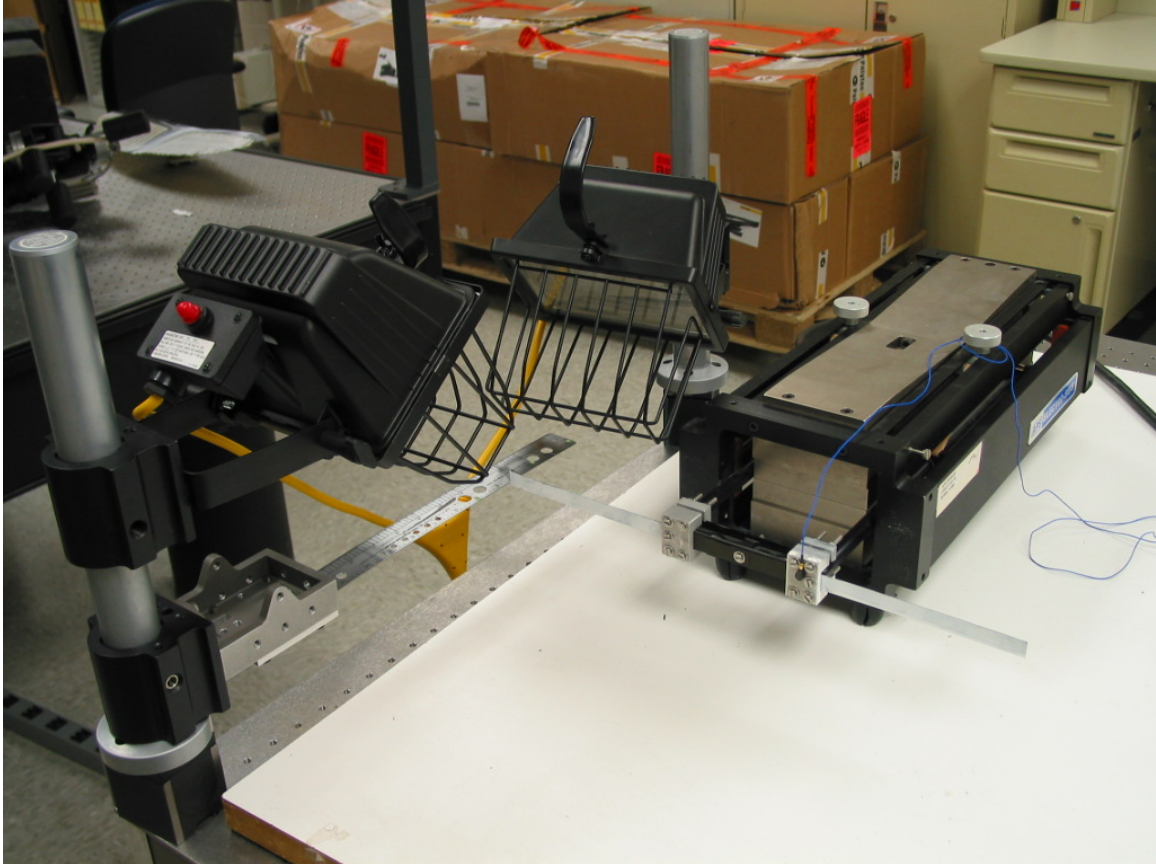
Figure 26: Test Stands, Spotlights, and Ruler Setup for High Speed Testing
