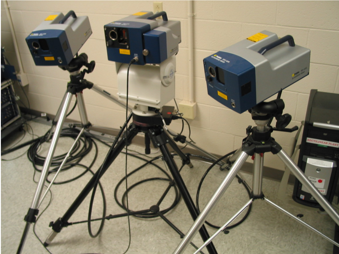
Figure 28: Right, Center, and Left PSV-400 Scanning Heads
