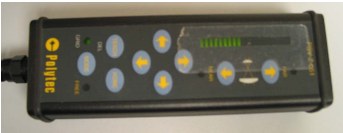
Figure 34: 3-D Alignment Remote Control
