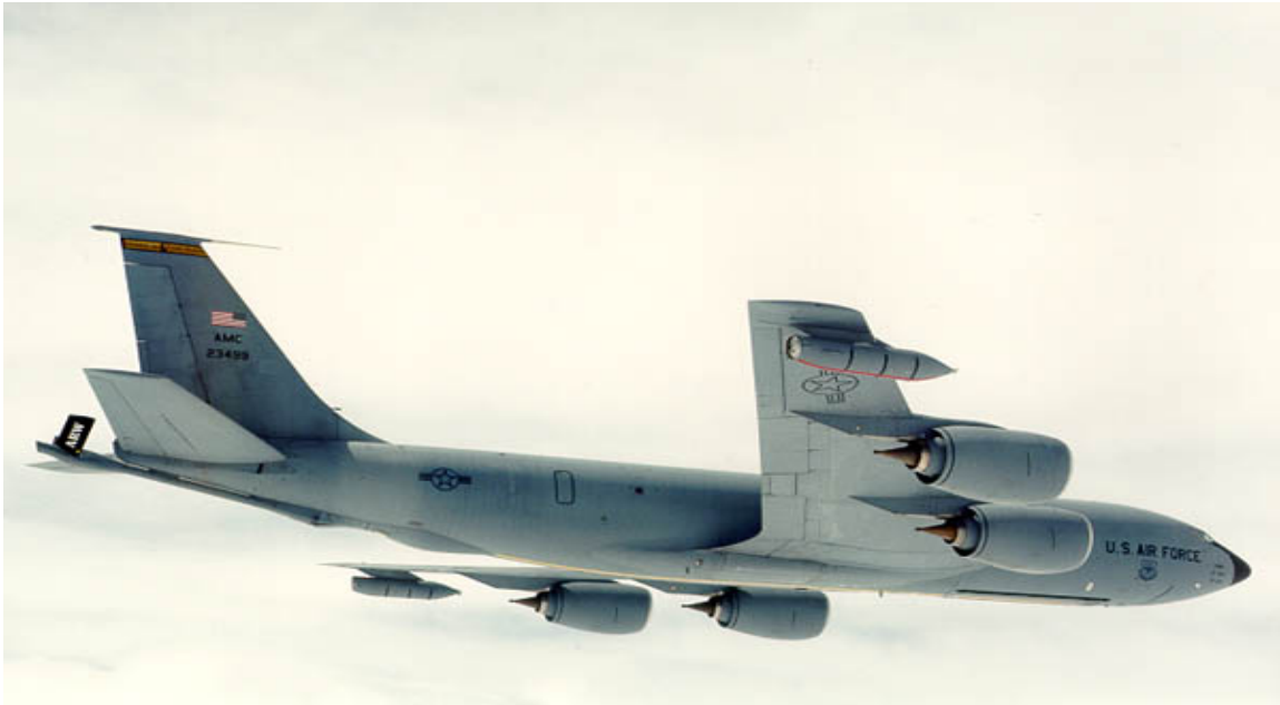
Figure 1. USAF KC-135 Stratotanker with Flying Boom in the Stowed Position (3).
