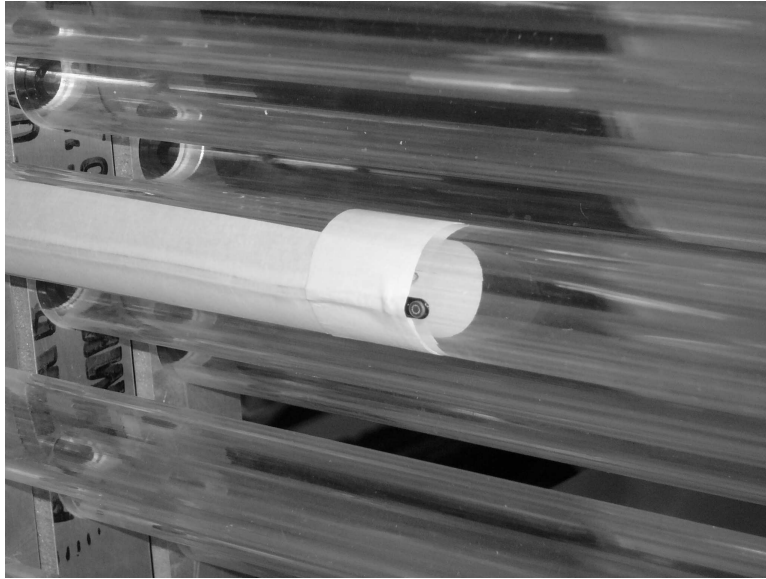
Figure 3.9: Photograph of the 5psig pressure transducer flush mounted to the front-center cylinder.
