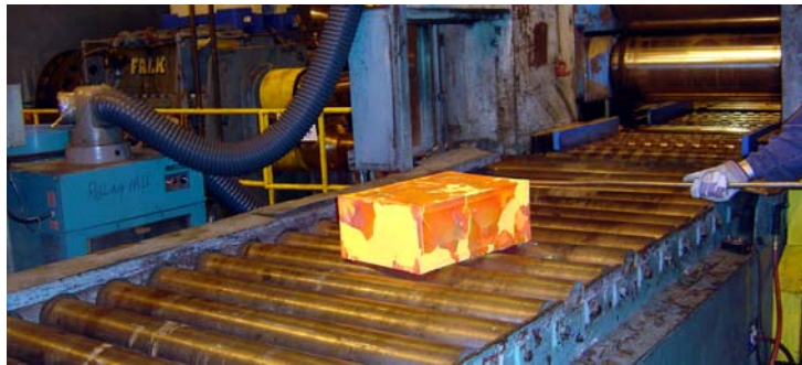
Figure 3.6: Ti64+1B billet just transferred from furnace to rolling mill. Ref: Tamirisakandala.
