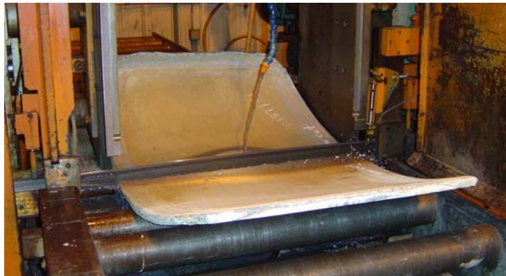
Figure 3.10: Cutting Ti64+1B rolled plate into two plates. Ref: Tamirisakandala.
