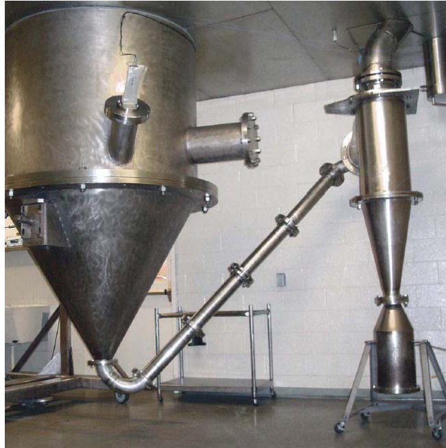
Figure 3.1: Picture of titanium atomization tower and cyclone at Crucible Research Corporation used to make Ti64+1B powder via pre-alloyed approach. Ref: Yolton, 2007 TMS presentation.
