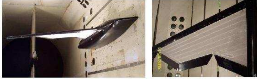
Figure 1.2: Front and top views of N-MAS model in the NASA LaRC transonic wind tunnel [13].
