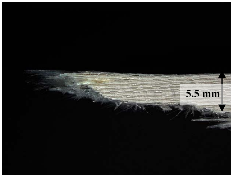
Figure 192. Fracture surface of N720/A specimen tested in compressive creep at -60 MPa for 100 h at 1200°C in air.
