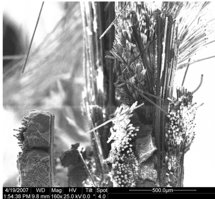
Figure 94. Fracture surface of N720/A specimen tested in creep at 60 MPa in air at 1200°C.
