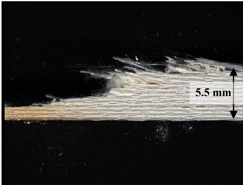
Figure 181. Fracture surface of N720/A specimen tested in compressive creep at -100 MPa for 100 h at 1200°C in air.
