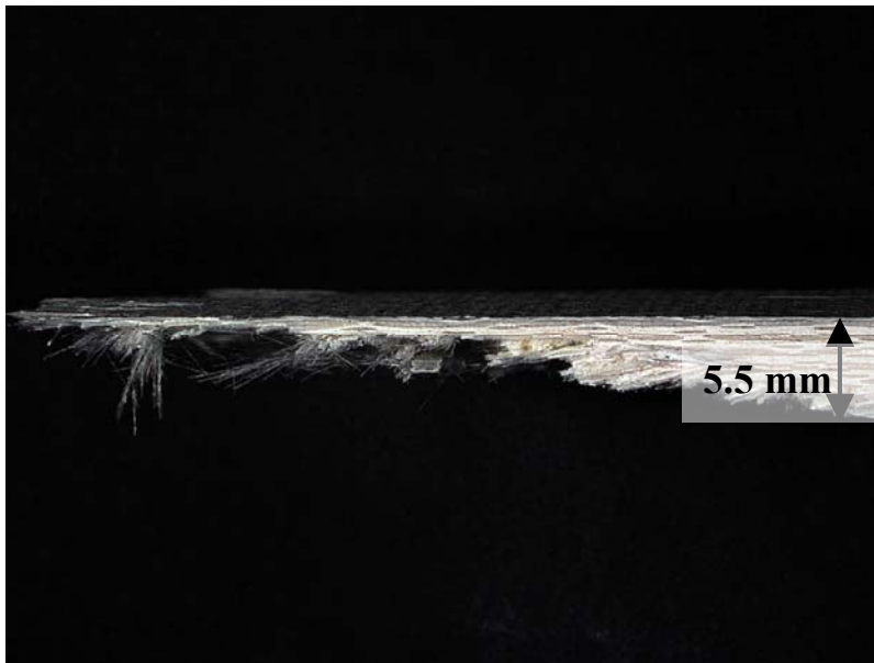
Figure 176. Fracture surface of N720/A specimen tested in compression to failure in displacement control at a rate of -0.05 mm/s in air at 1200°C.
