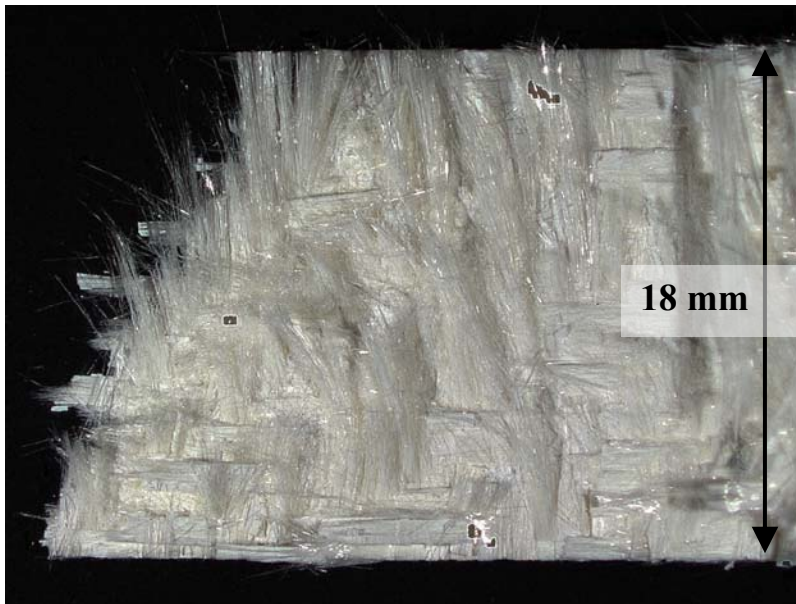
Figure 178. Fracture surface of N720/A specimen tested in compressive creep at -100 MPa for 100 h at 1200°C in air.
