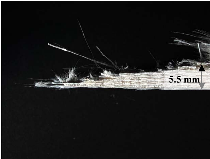
Figure 189. Fracture surface of N720/A specimen tested in compressive creep at -60 MPa for 100 h at 1200°C in air.
