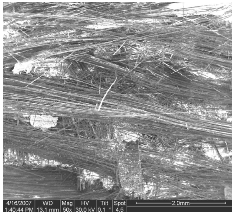
Figure 53. Fracture surface of N720/A specimen tested in compression to failure in displacement control at a rate of -0.05 mm/s in steam at 1200°C.
