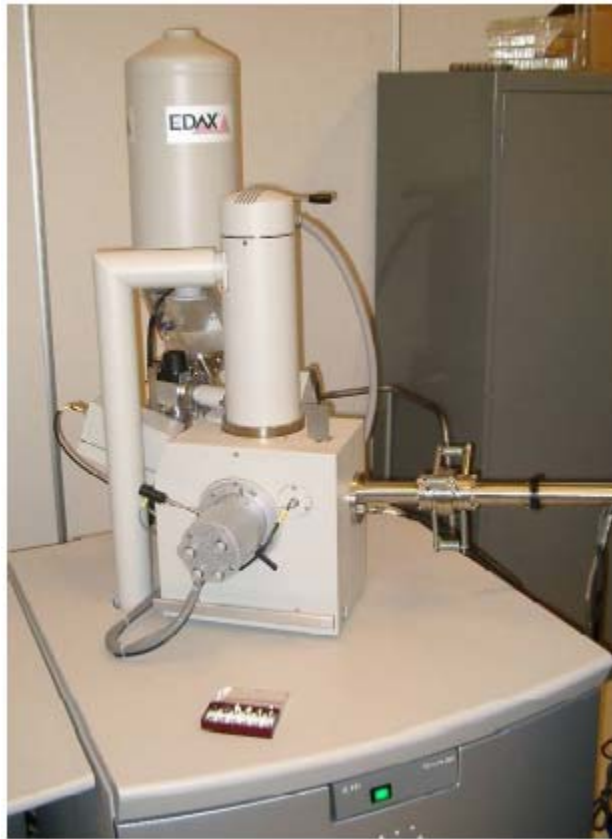
Figure 22. FEI Quanta Scanning Electron Microscope (SEM) and EDAX X-Ray Analysis System.
