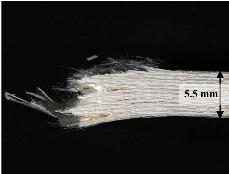
Figure 219. Fracture surface of N720/A specimen subjected to aging in steam at 1200°C for 25 h then failed in compression.
