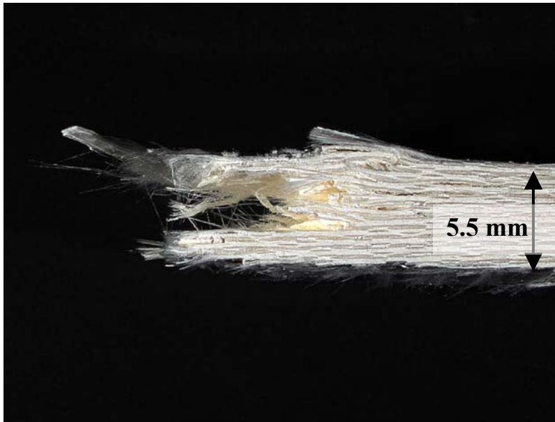
Figure 229. Fracture surface of N720/A specimen tested in compression to failure in steam at 1200°C in displacement control at -0.05 mm/s.
