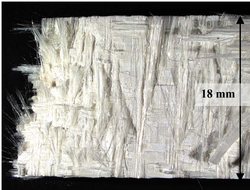
Figure 190. Fracture surface of N720/A specimen tested in compressive creep at -60 MPa for 100 h at 1200°C in air.
