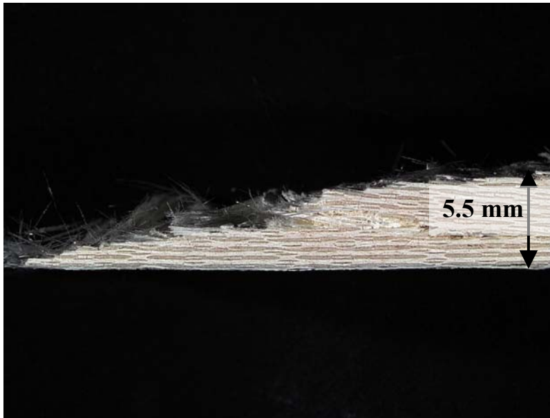
Figure 175. Fracture surface of N720/A specimen tested in compression to failure in displacement control at a rate of -0.05 mm/s in air at 1200°C.
