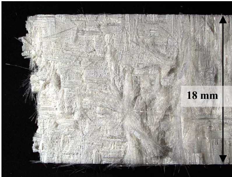
Figure 231. Fracture surface of N720/A specimen tested in compression to failure in air at 1200°C in stress control at -0.0025 MPa/s.
