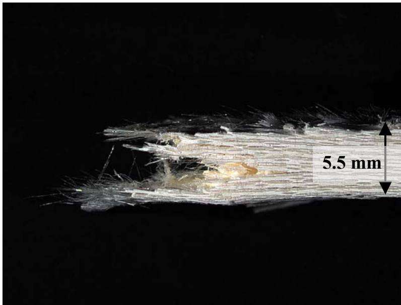
Figure 222. Fracture surface of N720/A specimen tested in compression to failure in steam at 1200°C in displacement control at -0.05 mm/s.
