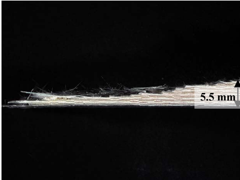
Figure 169. Fracture surface of N720/A specimen tested in compression to failure in displacement control at a rate of -0.05 mm/s in air at 1200^{\circ}\text{C} .
