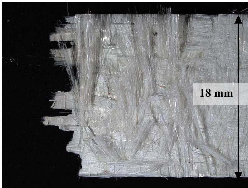
Figure 170. Fracture surface of N720/A specimen tested in compression to failure in displacement control at a rate of -0.05 mm/s in air at 1200^{\circ}\text{C} .
