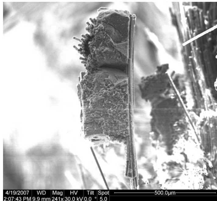
Figure 99. Fracture surface of N720/A specimen tested in creep at 60 MPa in air at 1200°C.
