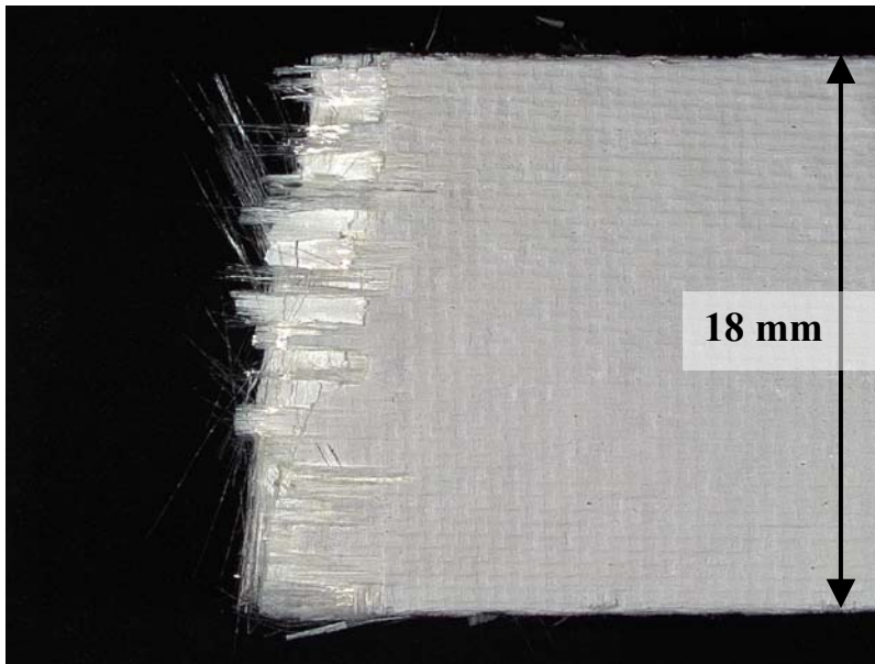
Figure 220. Fracture surface of N720/A specimen subjected to aging in steam at 1200°C for 25 h then failed in compression.
