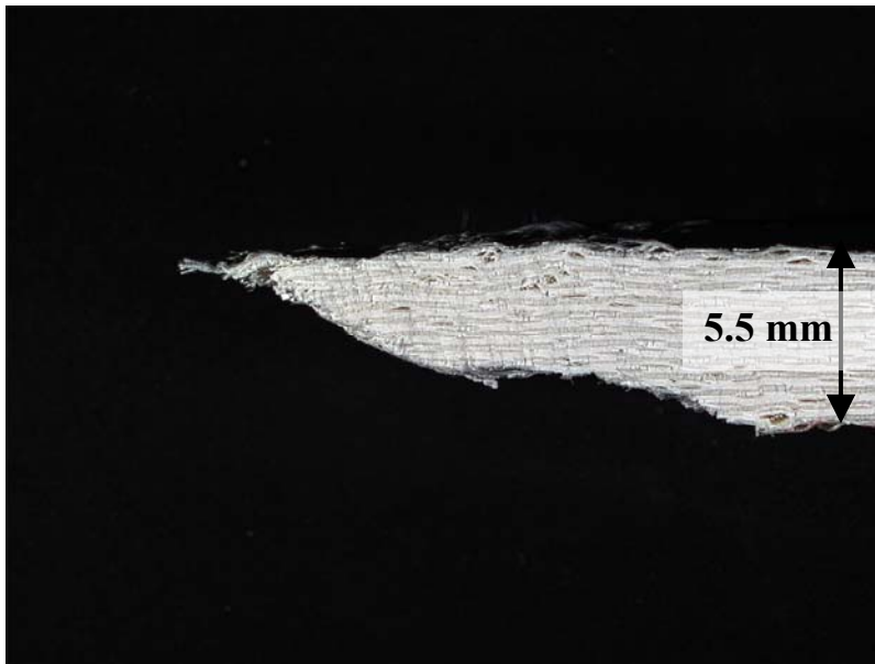
Figure 210. Fracture surface of N720/A specimen tested in compressive creep at -40 MPa for 100 h at 1200°C in steam.
