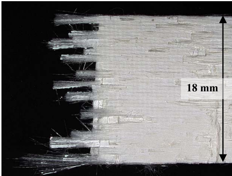
Figure 195. Fracture surface of N720/A specimen tested in compressive creep at -100 MPa for 100 h at 1200°C in steam.
