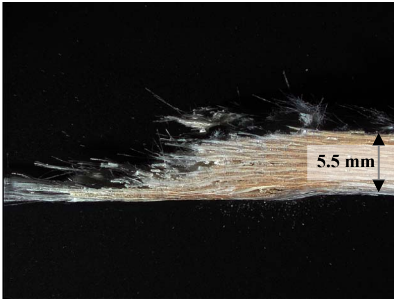
Figure 183. Fracture surface of N720/A specimen tested in compressive creep at -100 MPa for 100 h at 1200°C in air.
