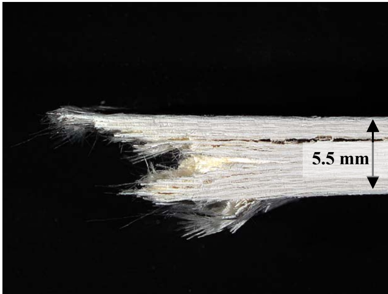
Figure 221. Fracture surface of N720/A specimen subjected to aging in steam at 1200°C for 25 h then failed in compression.
