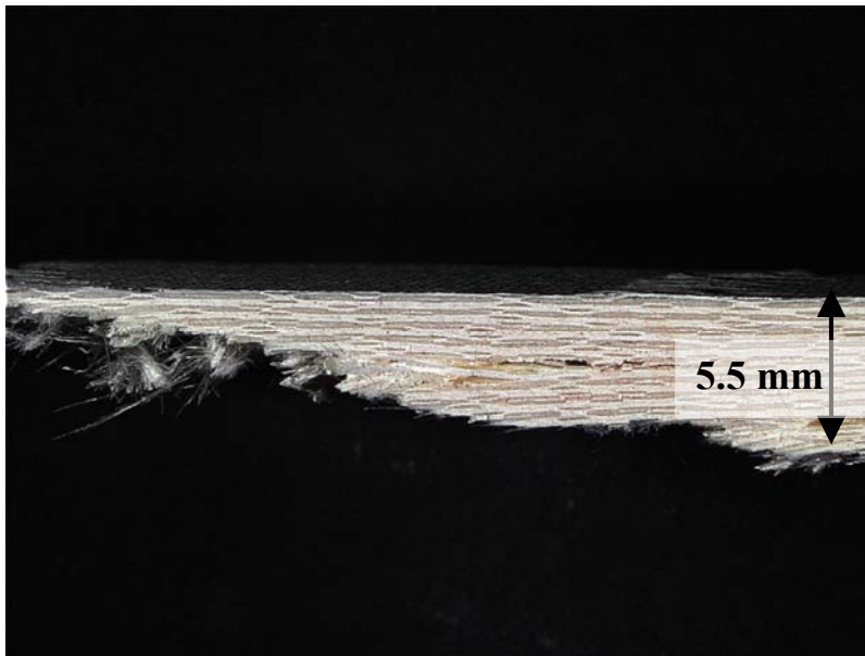
Figure 174. Fracture surface of N720/A specimen tested in compression to failure in displacement control at a rate of -0.05 mm/s in air at 1200°C.
