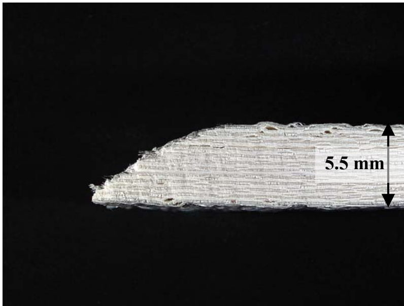
Figure 240. Fracture surface of N720/A specimen tested in compression to failure in steam at 1200°C in stress control at -0.0025 MPa/s.
