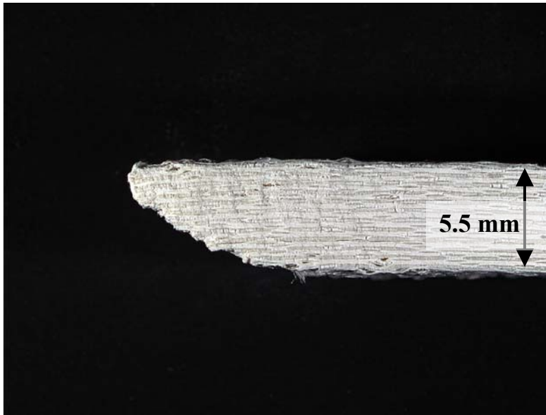
Figure 239. Fracture surface of N720/A specimen tested in compression to failure in steam at 1200°C in stress control at -0.0025 MPa/s.
