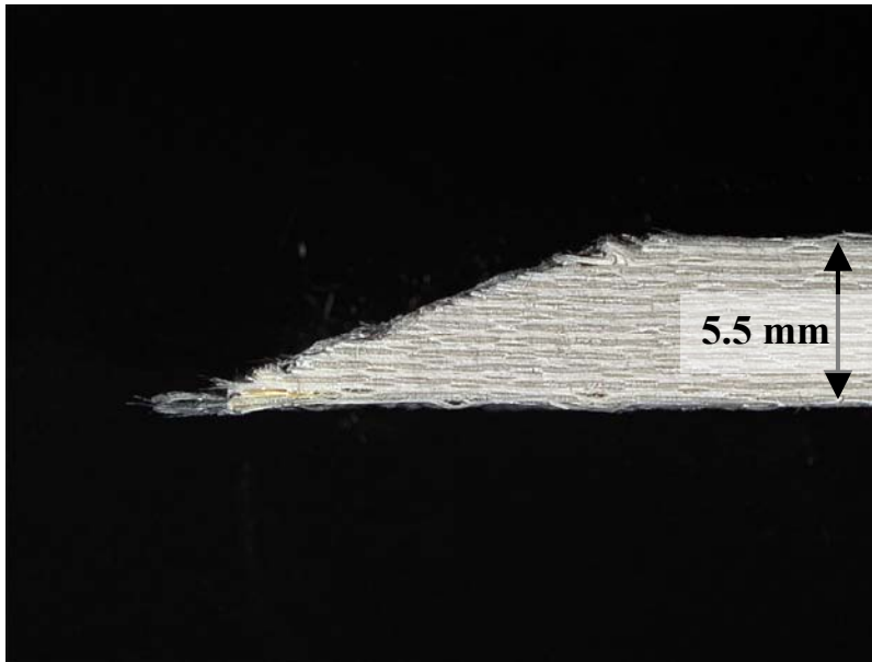
Figure 199. Fracture surface of N720/A specimen tested in compressive creep at -60 MPa for 100 h at 1200°C in steam.
