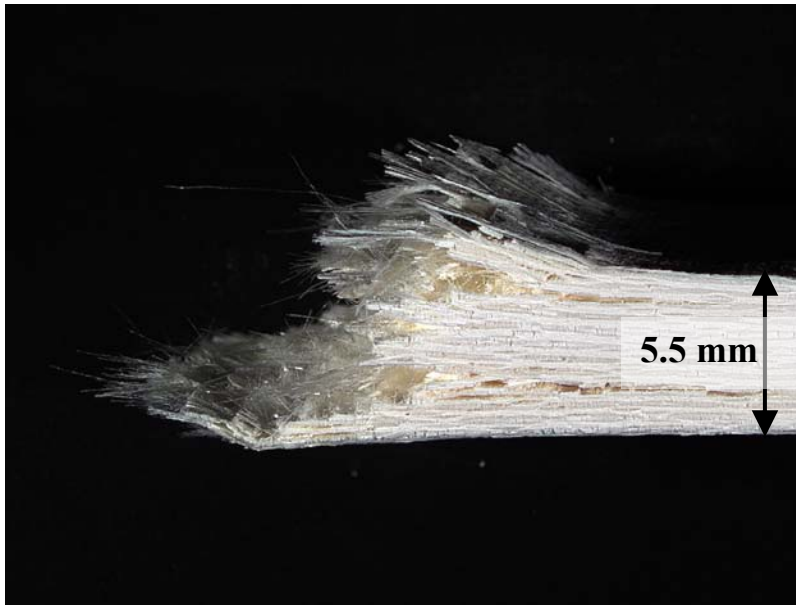
Figure 215. Fracture surface of N720/A specimen subjected to aging in steam at 1200°C for 25 h then failed in compression.
