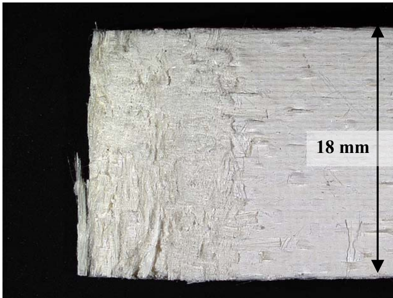
Figure 200. Fracture surface of N720/A specimen tested in compressive creep at -60 MPa for 100 h at 1200°C in steam.
