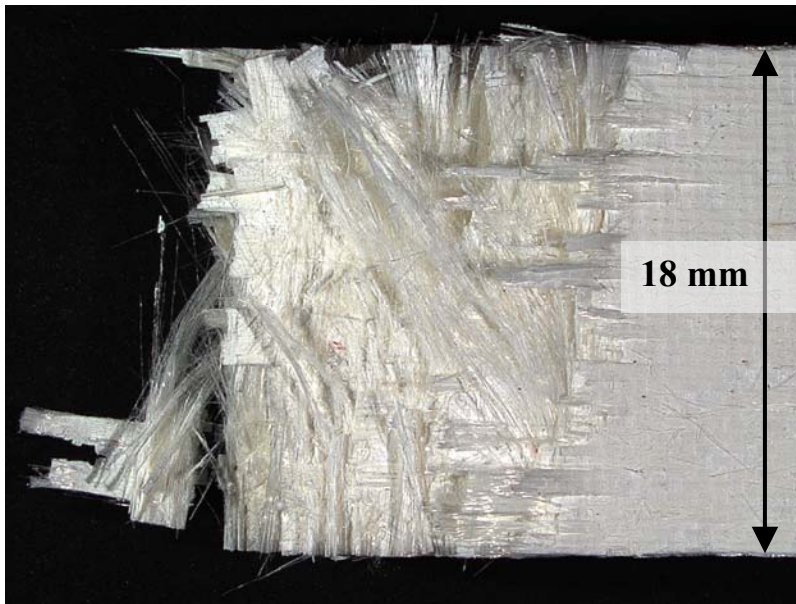
Figure 216. Fracture surface of N720/A specimen subjected to aging in steam at 1200°C for 25 h then failed in compression.
