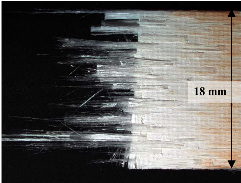
Figure 177. Fracture surface of N720/A specimen tested in compressive creep at -100 MPa for 100 h at 1200°C in air.
