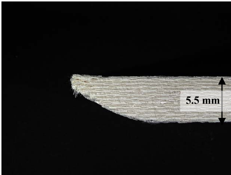
Figure 202. Fracture surface of N720/A specimen tested in compressive creep at -60 MPa for 100 h at 1200°C in steam.
