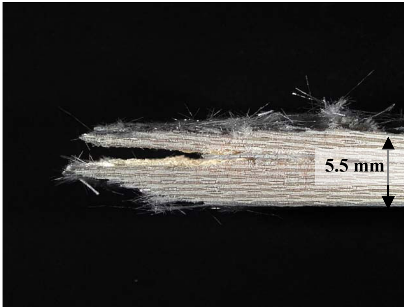
Figure 233. Fracture surface of N720/A specimen tested in compression to failure in air at 1200°C in stress control at -0.0025 MPa/s.
