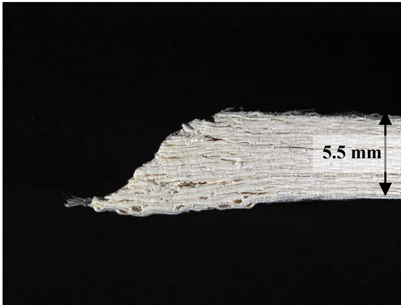
Figure 213. Fracture surface of N720/A specimen tested in compressive creep at -40 MPa for 100 h at 1200°C in steam.
