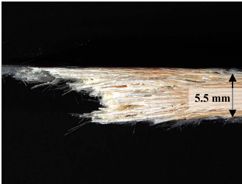
Figure 182. Fracture surface of N720/A specimen tested in compressive creep at -100 MPa for 100 h at 1200°C in air.
