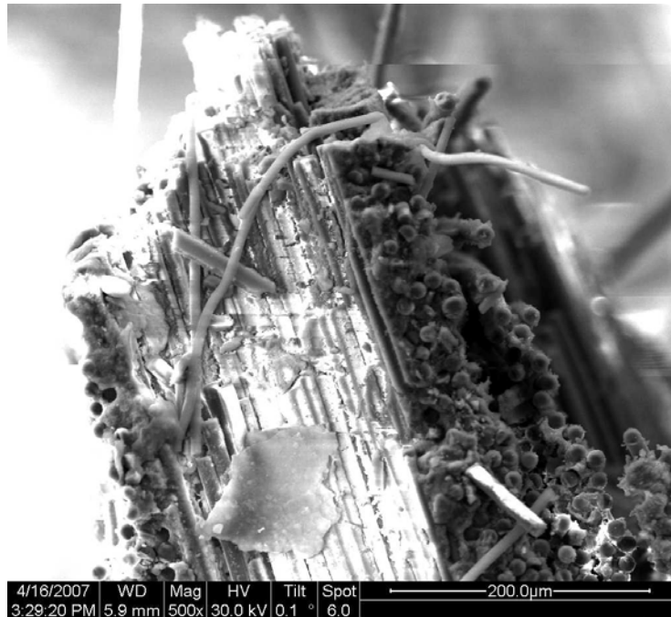
Figure 74. Fracture surface of N720/A specimen tested in compression to failure in displacement control at a rate of -0.05 mm/s in steam at 1200°C.
