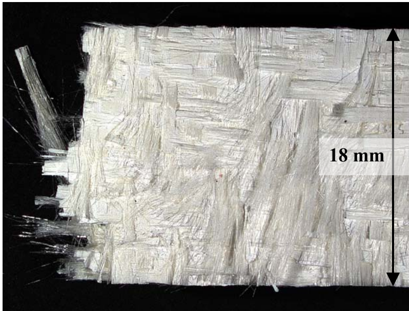
Figure 227. Fracture surface of N720/A specimen tested in compression to failure in steam at 1200°C in displacement control at -0.05 mm/s.
