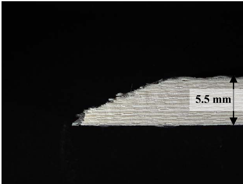
Figure 203. Fracture surface of N720/A specimen tested in compressive creep at -60 MPa for 100 h at 1200°C in steam.
