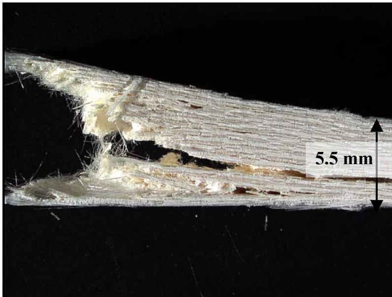
Figure 196. Fracture surface of N720/A specimen tested in compressive creep at -100 MPa for 100 h at 1200°C in steam.
