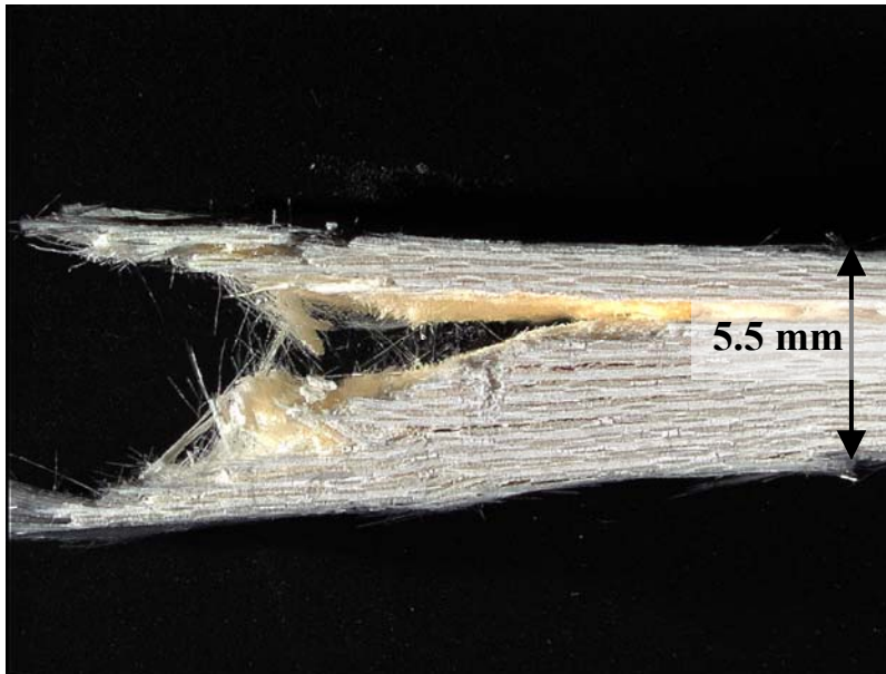
Figure 197. Fracture surface of N720/A specimen tested in compressive creep at -100 MPa for 100 h at 1200°C in steam.
