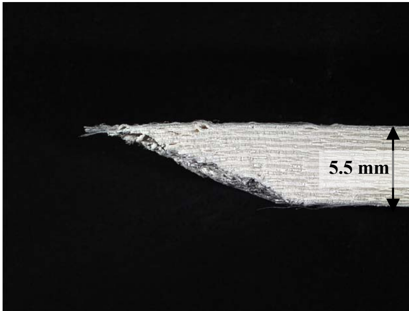
Figure 243. Fracture surface of N720/A specimen tested in compression to failure in steam at 1200°C in stress control at -0.0025 MPa/s.
