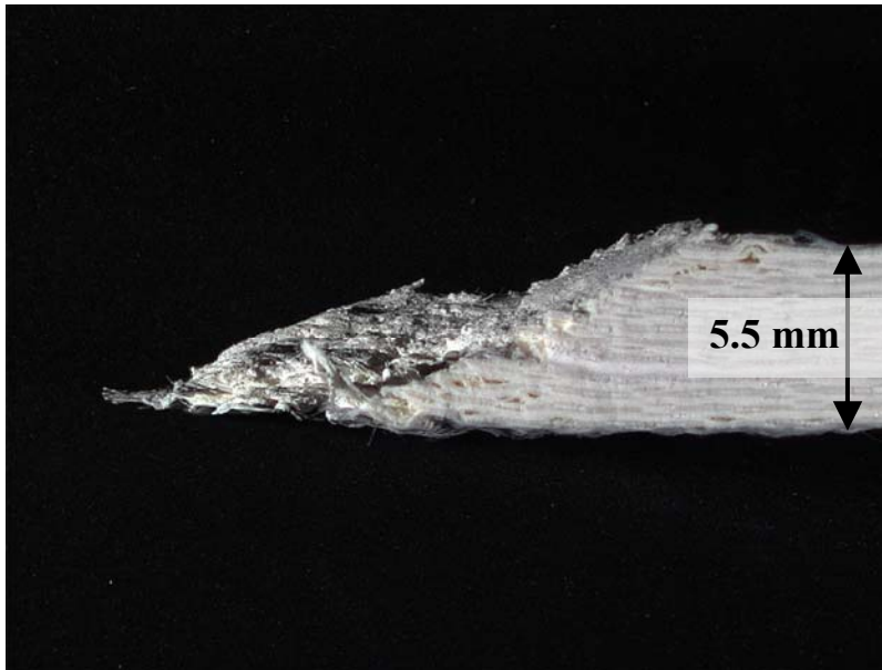
Figure 211. Fracture surface of N720/A specimen tested in compressive creep at -40 MPa for 100 h at 1200°C in steam.
