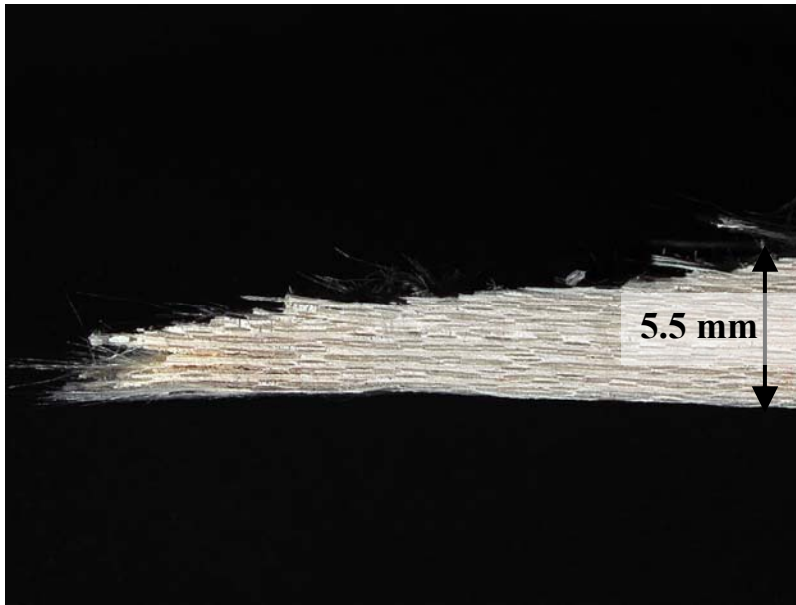
Figure 185. Fracture surface of N720/A specimen tested in compressive creep at -60 MPa for 100 h at 1200°C in air.
