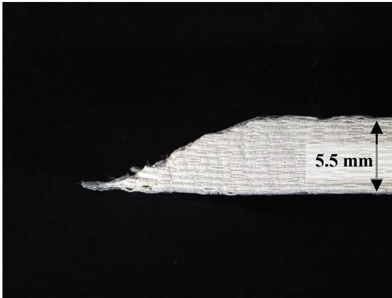
Figure 237. Fracture surface of N720/A specimen tested in compression to failure in steam at 1200°C in stress control at -0.0025 MPa/s.
