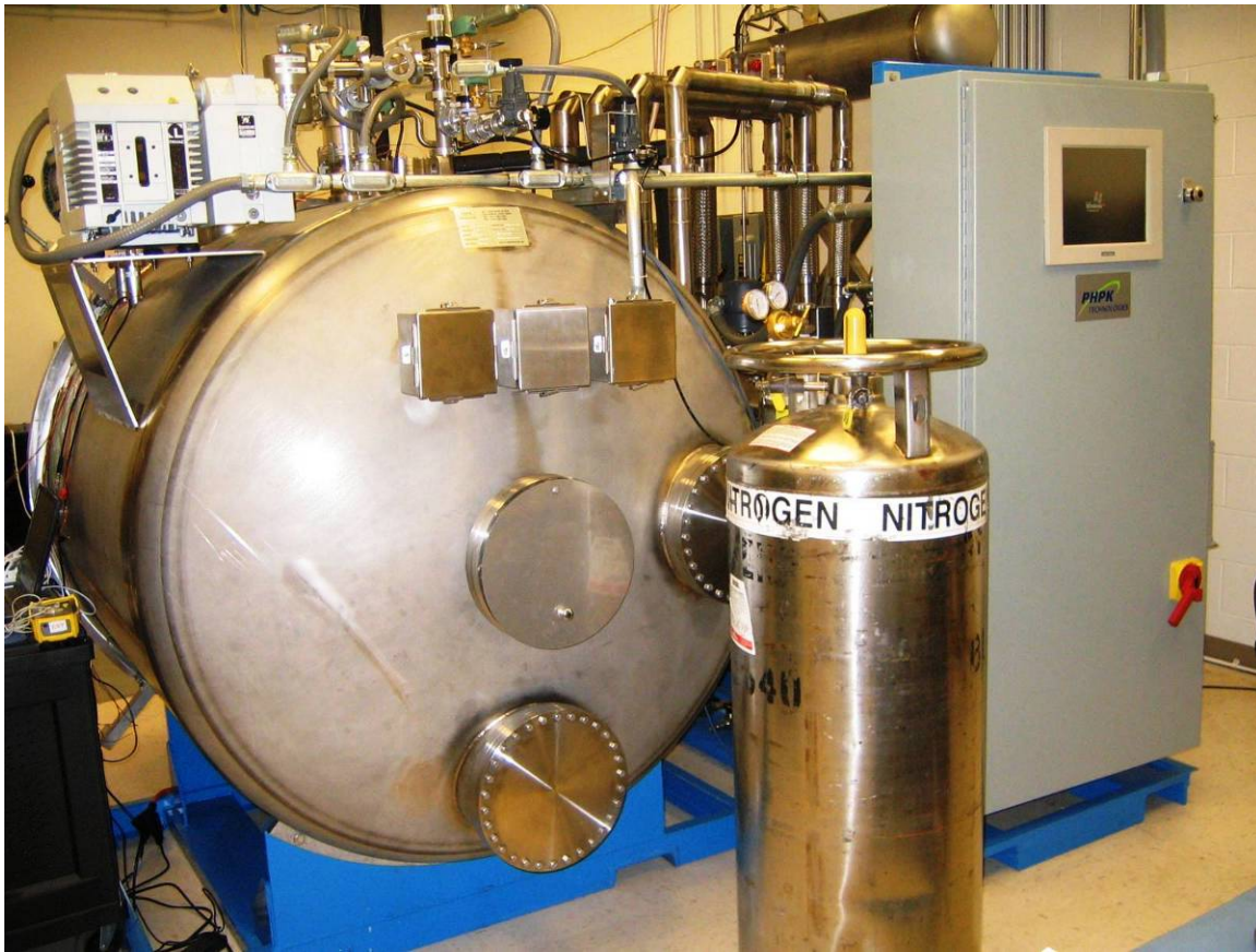
Figure 28: AFIT TVAC Chamber Rear Control Panel.
