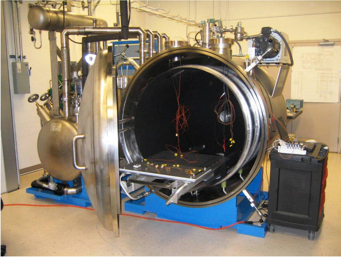
Figure 26: AFIT TVAC Platen Pulled Open to Access Test Panel.
