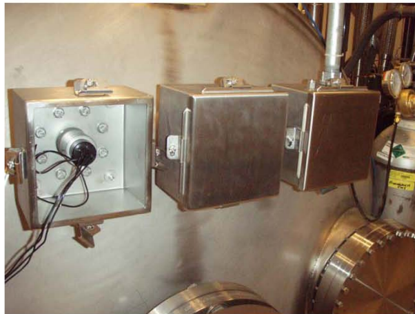
Figure 30: Connection of Emulators Wires to Rear Wiring Interface Outside Chamber
