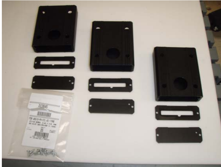
Figure III-32: Aluminum Enclosures after Being Anodized
