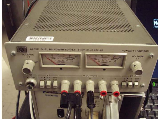
Figure 33: Connection of Wires to DC Power Supply
