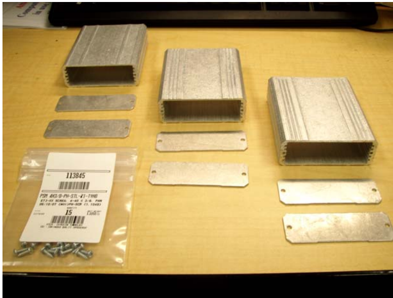
Figure III-30: Aluminum Enclosures with Blank Endplates and Extrusions
