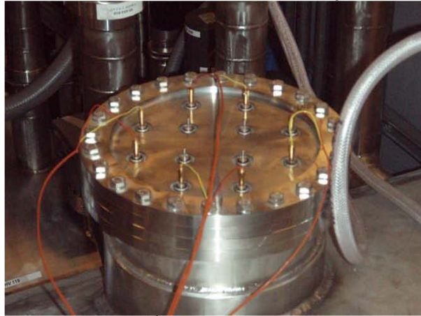
Figure 29: Connection of 2 nd Set of Thermocouple Wires to Right Wiring Interface Outside Chamber
