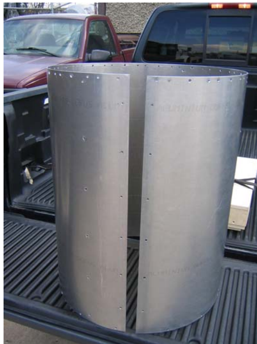
Figure V-4: Final Design of Seam
