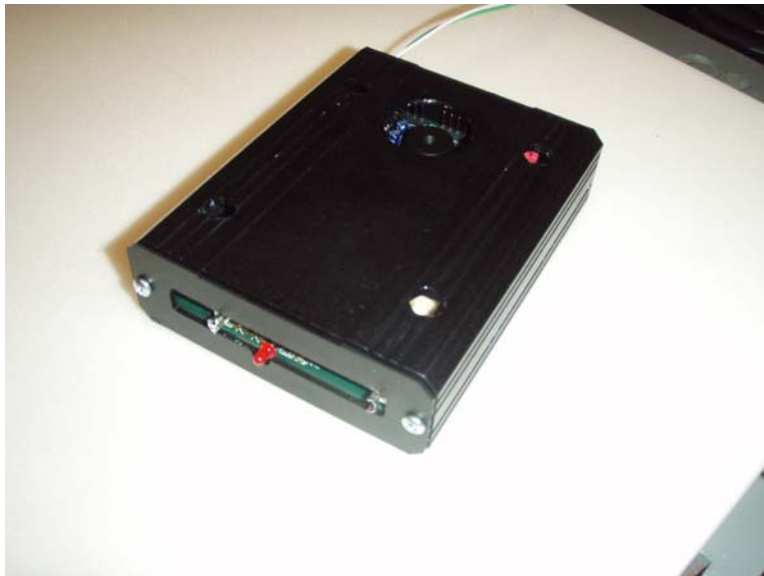
Figure III-33: Aluminum Enclosure Assembled Together with Eye-C Inside
