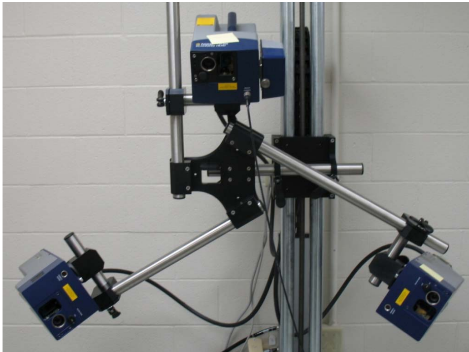
Figure 5: PSV-I-400 Scanning Heads on Motorized Tripod
