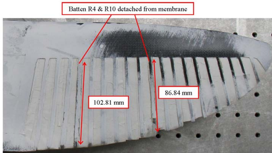
Figure 15: Test 1, Right Span Wing Damage
