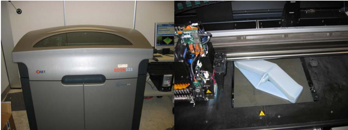
Figure 44: The Objet Eden 333 Printer and the Printer Head during the Build Process
