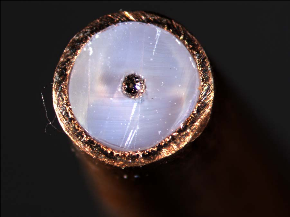
Figure 51 - Flat tip of an unused propellant tube
