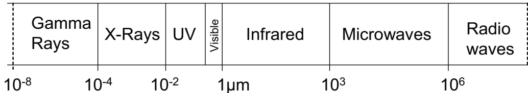
Figure 1.1: The infrared spectrum is a subset of the electromagnetic spectrum. Wavelength is in units of microns ( \mu\text{m} ). Adapted from [4, Figure 1.1].
