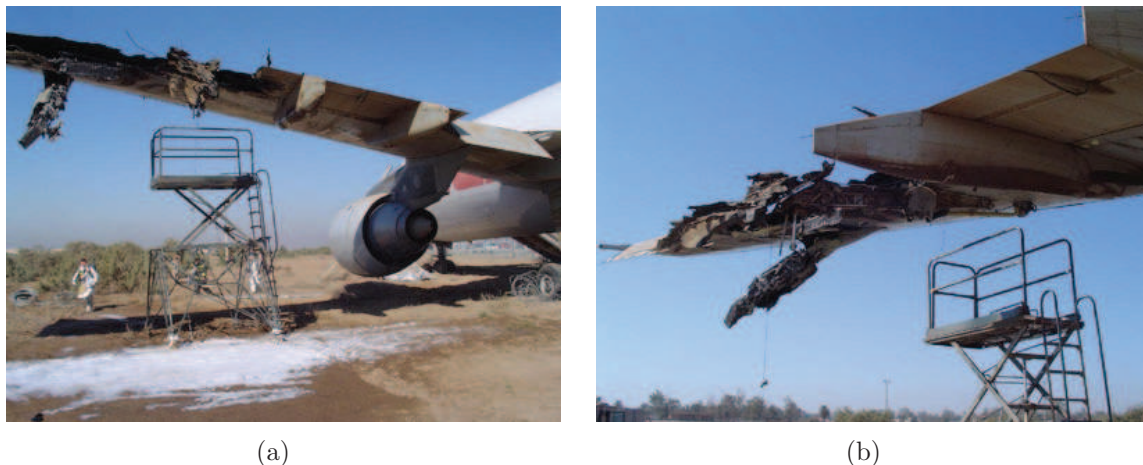
Figure 1.2: The DHL A330 aircraft was hit by an SA-14 MANPADS in the left wing and lost all hydraulics. Reproduced from airdisaster.com .
