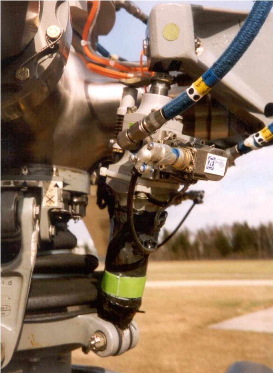
Figure 2.7: Individual Dynamic Pitch Linkage on a BO 105 [20].
