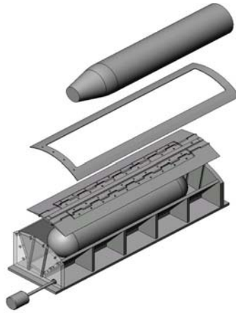
Figure 2-9: Naval Bomb Bay Ejector Airbag Test Apparatus (with permission of authors [2-16])
