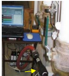
Figure 5-3: Hose, Valve, and Fittings
