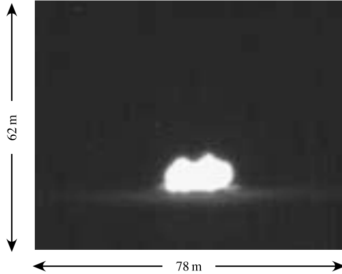
Figure 23: Image captured by the Alpha NIR FPA ( 320 \times 256 ) during the detonation of 50 kg of TNT. The square root of the fireball area, defined by the number of saturated pixels, is approximately 10.5 m.
