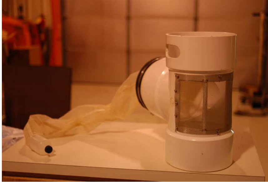
Figure 13. Modified Hess Sampler Used to Sample Treatment Areas.
