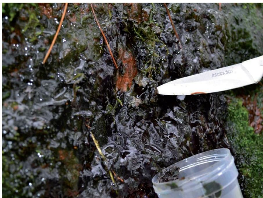
Figure 5. Biofilm formed by the cyanobacteria from the genera Lyngbya and Synechococcus on a granite wall in Monrepos Park (Vyborg).
