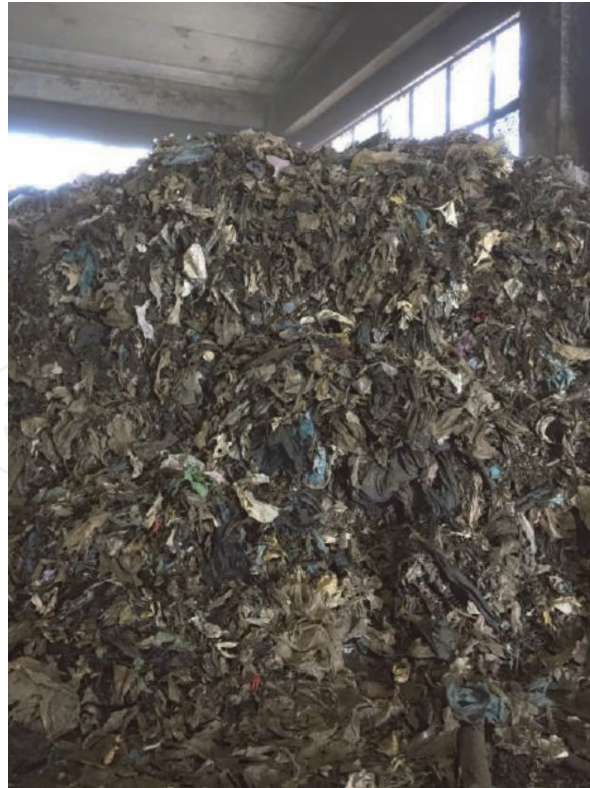
Figure 2. Waste removed by the biowaste in the pretreatment stage.
