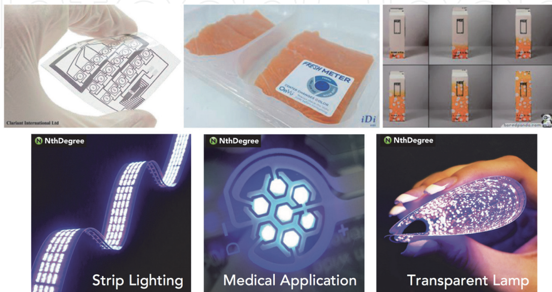
Figure 9. Printed electronics samples: circuit printed with nano-silver ink [35], printed sensor that shows food spoilage [36], smart box packaging that enables end-of-life display by color change [37], and various lighting applications [38].
