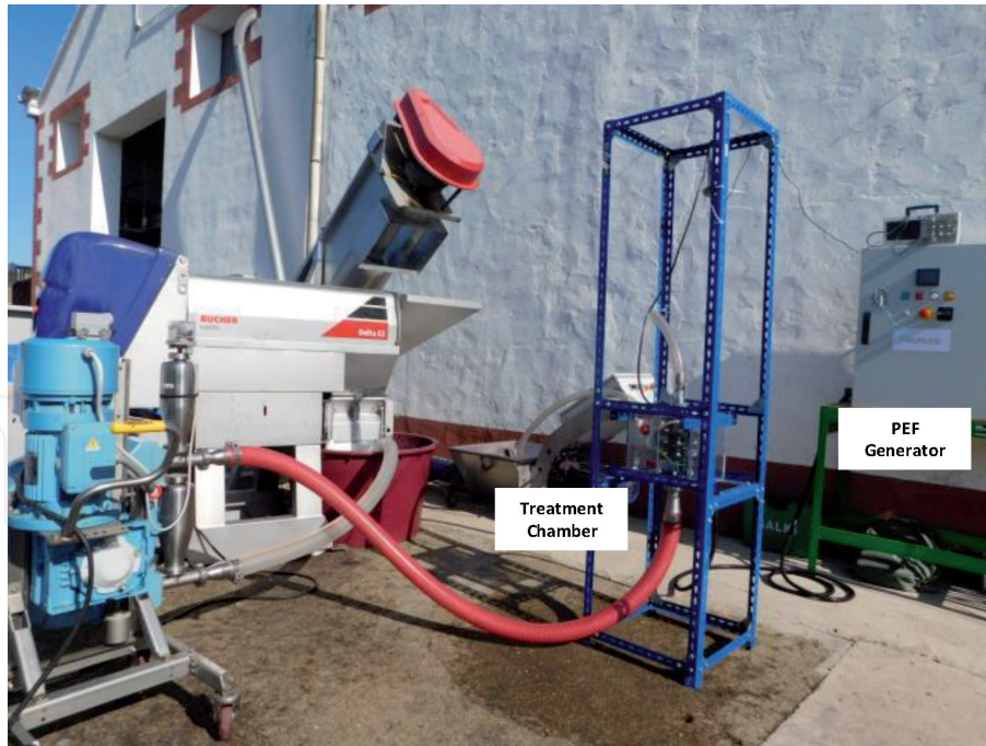
Figure 9. PEF experimental unit to process the crushed grapes at a flow of 3 t/h to improve the polyphenols extraction in the maceration-fermentation stage of red winemaking.
