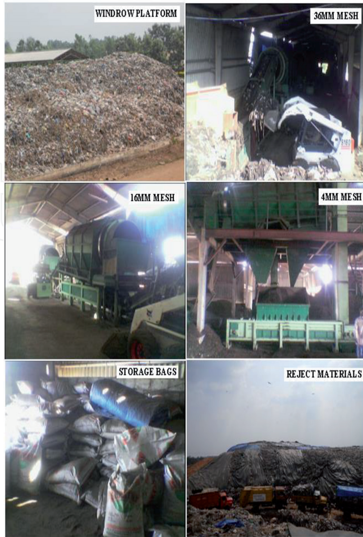
Figure 8. Windrow composting process.
