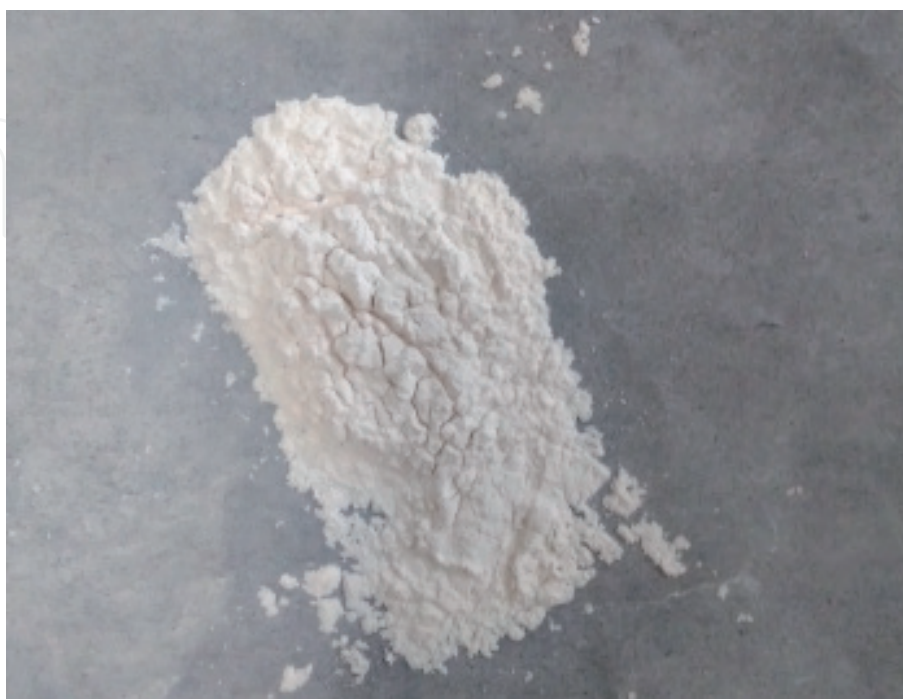
Figure 8. P molecular sieve prepared by coal fly ash.
