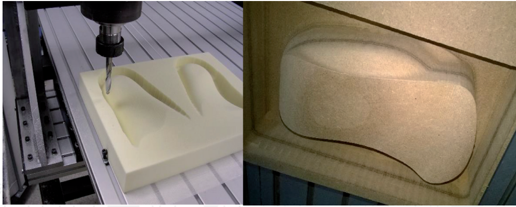
Figure 4. Molds for foot orthoses production.
