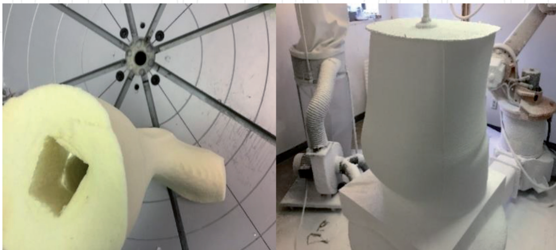
Figure 15. Molds produced from expanded PU foam.
