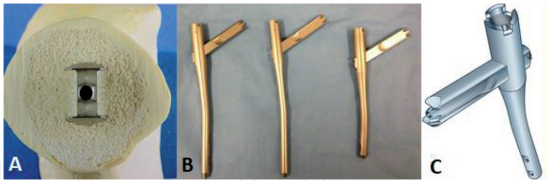
Figure 6. (A) Axial view of the double-T blade profile inside the femoral head (sawbone); (B) lateral view of the GN in three sizes; and (C) 3D view of the gliding nail.
