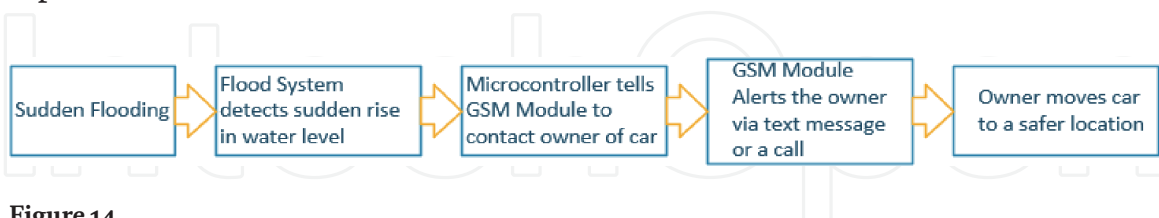
Figure 14. Diagram of the process for a flood alert system.
