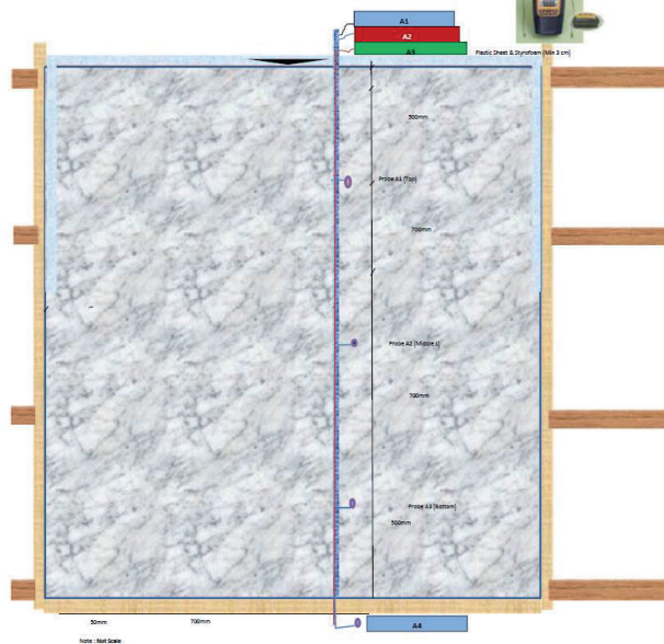
Figure 19. Thermocouple Bioconc-LHC monitoring, Summary data & mock up sketch.
