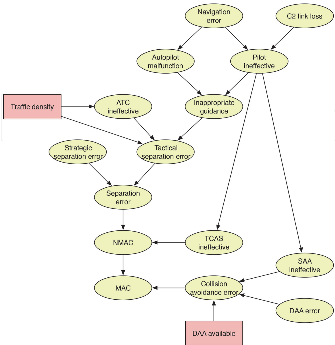
Figure 5. Mid-air collision BBN model in controlled airspace.
