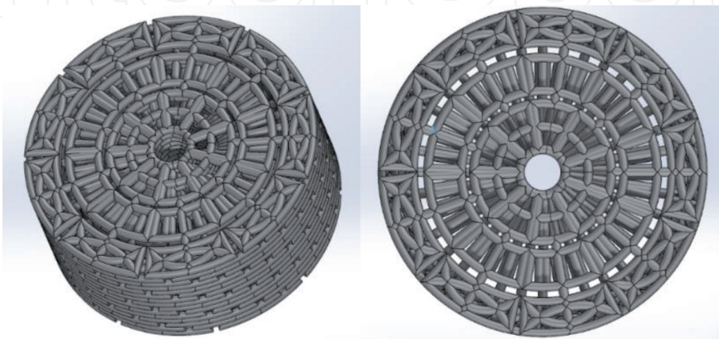
Figure 6. DNA chain-inspired cylindrical scaffold.
