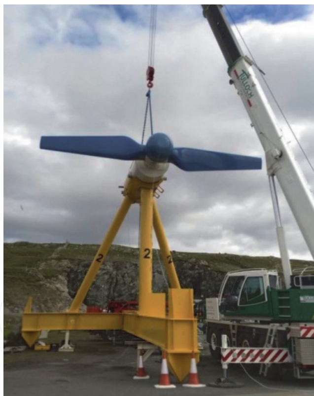
Figure 2. Nova M100 tidal turbine (Source: ©Nova Innovation).
