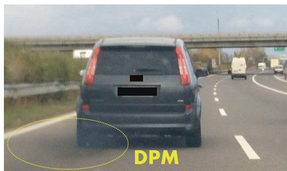
Figure 1. Black cloud of particulate matter and soot exhaust emissions from the tail pipe of on-road diesel engine passenger vehicle.
