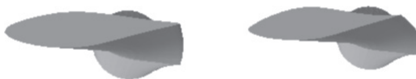
Figure 6. Top view of the blade with S809gx (left) and S809 (right).
