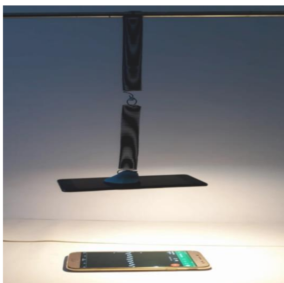
Figure 5. The photography of the serial connected spring-mass system.
