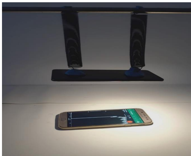
Figure 7. The photography of the parallel connected spring-mass system with two smartphones.
