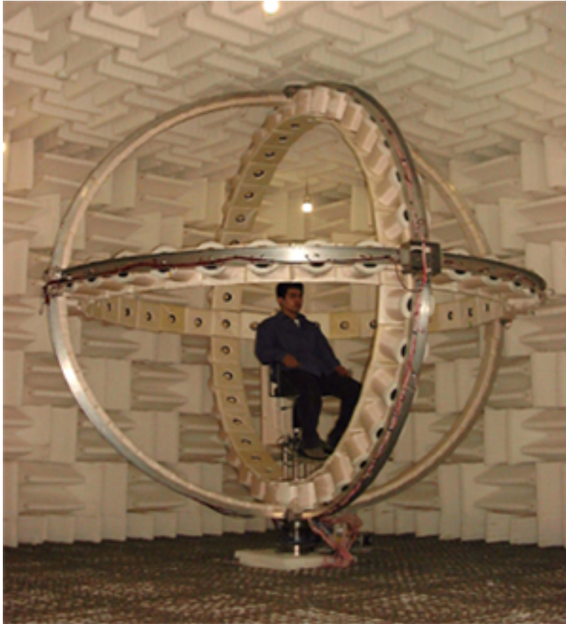
Figure 1.2: Loudspeaker array for measuring HRTF in Tohoku University.
