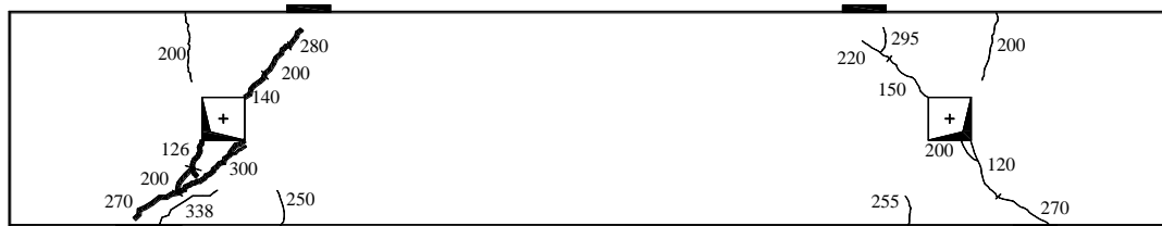
(a) schematic drawing of the crack pattern
