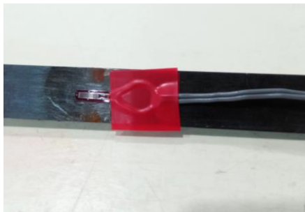
(a) Strain gauge attached on CFRP strip
