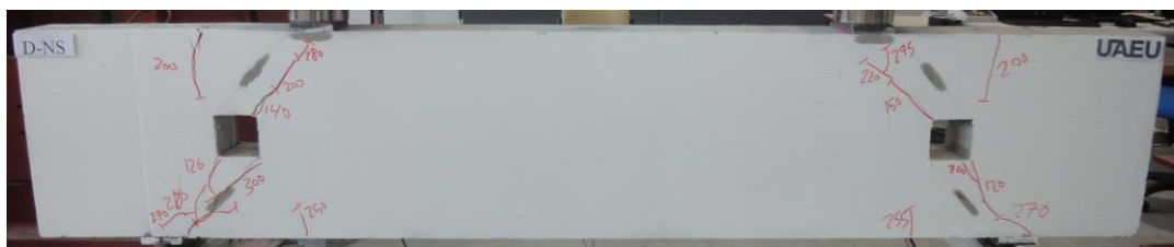
(b) picture of the beam at failure
