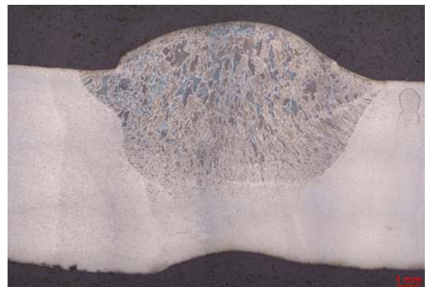
Figure 7: Sample B3 — capping layer, short arc 145 A
