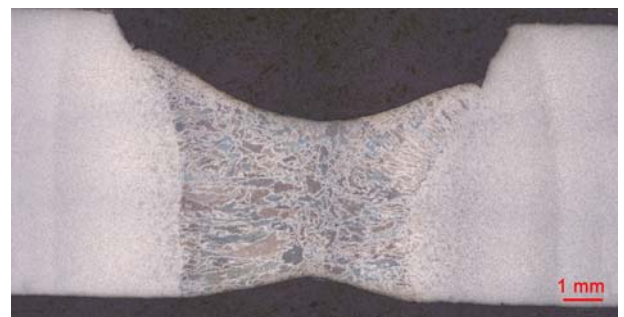
Figure 6: Sample B3 — root weld, short arc 130 A
