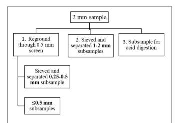
**FIGURE 1** | Schematic of subsampling of 2 mm samples into different particle sizes. 2 mm particle sized samples were obtained by grinding dried samples and allowed to pass through 2 mm screen of a cyclone mill.
