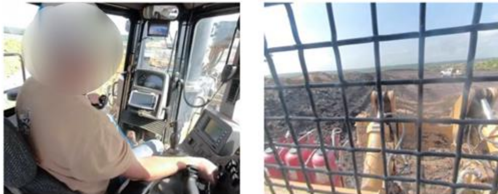
Figure 20 - Camera Position for SVP Videos for Dozers
