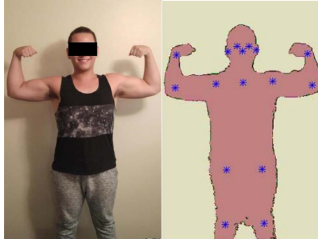
Figure 2.5: The body contour and skeleton-joints detected by the CSJ detector. The brick red area represent the detected body part. The asterisks represents the skeleton joints.
