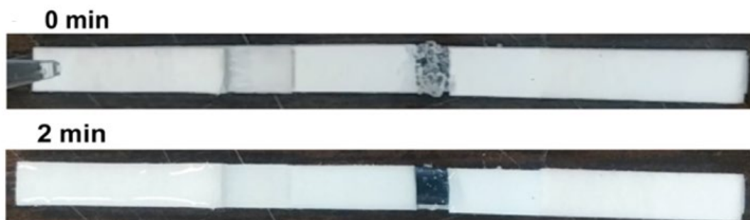
Figure 4.7. Optical images of a chip-PLFS before and after the sample solution is loaded.
