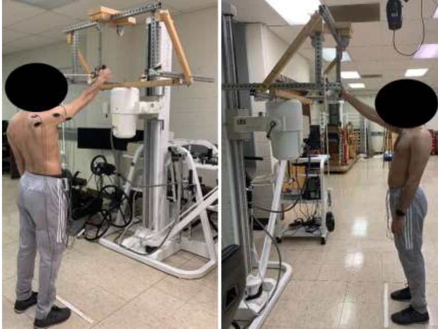
Figure 11: A participant performing a pull right (PR) direction while shoulder angle is elevated 120^\circ in the sagittal plane.
