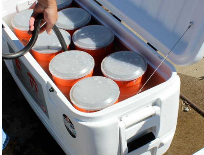
Figure 5-2: On-site curing of compressive strength specimens
