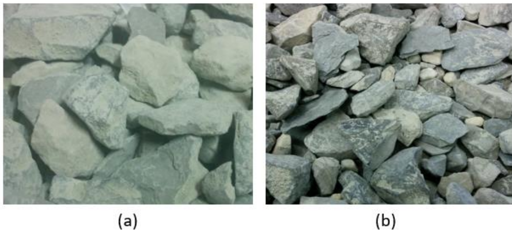
Figure 3-2: (a) Before washing with vinegar, (b) After washing with vinegar
