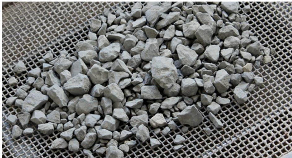
Figure 3-1: Large aggregate on sieve no. 4
