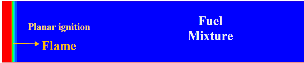
Figure 3.1: Schematic of a semi-open channel with smooth walls.
