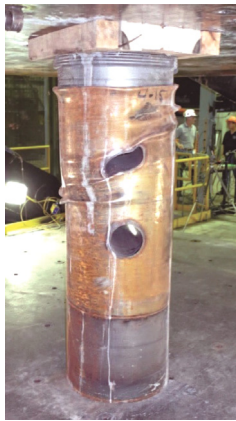
Fig. 6. The Eye CAN® with 45.72 cm vertical displacement (convergence), area of "eye" maintained.
