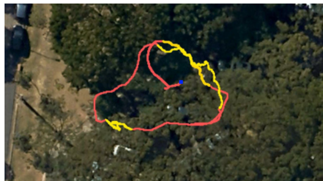
Figure 9. Satellite view of the forest where our experiments were executed. Image provided by Google Maps. The path estimated by RAUKF is shown in red whenever AHRS, LO, and GNSS were available and in yellow if only AHRS and LO were available. The vehicle's starting point is represented by the blue square.
