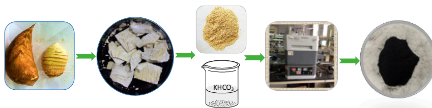
Figure 5. The preparation process of the nitrogen-doped carbon materials.
