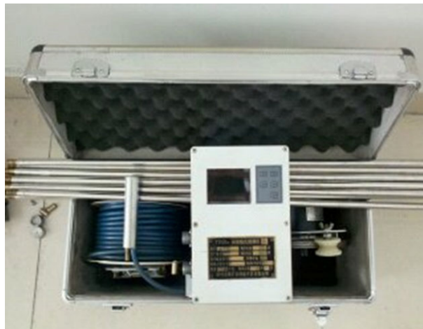
Figure 11. TYGD10 high-definition borehole camera detection.
