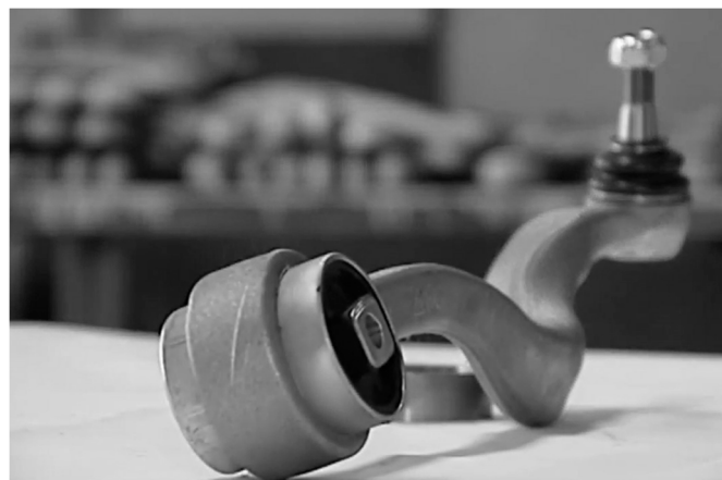
Figure 9. Suspension Control Arm remanufactured with Katok’s patented process © Katok.
