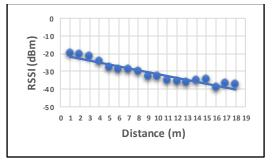
Fig. 6. Received Signal Strength to Distance
