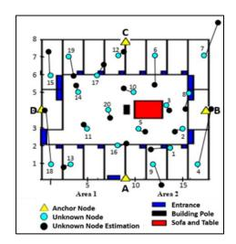
Fig. 7. Comparison Between Real Location and The Estimated Location of The Unknown Node
